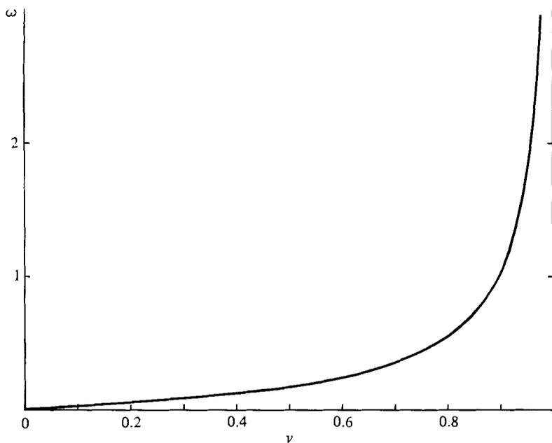
FIGURE 1. Vorticity distribution on the back face of the disk.
