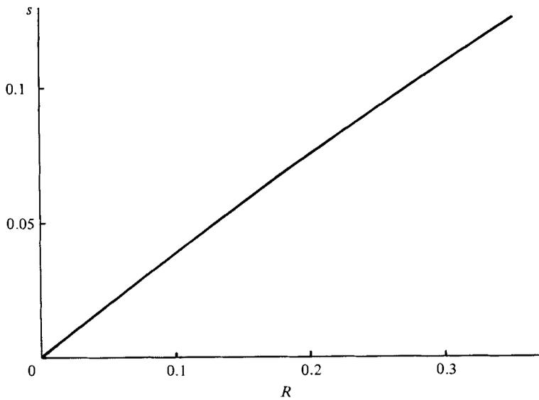
FIGURE 2. Size of standing vortex versus Reynolds number.
